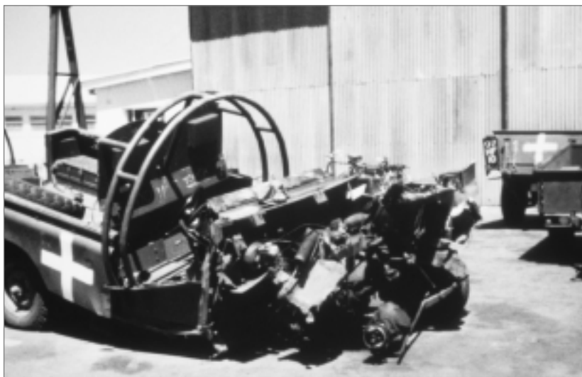
Southern Rhodesia. c. 1980. British Rover equipped with mine protection gear shows extensive damage from striking a mine. There were no casualties. The event was part of a peacekeeping operation by a contingent of 1300 men, including 150 Australians, sent to monitor elections.
